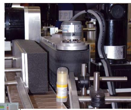
**LABEL APPLICATION.** The new labeler applies labels to Body Butter containers at speeds of approximately 30 per minute (above). Label-Aire's new Inline 6000 Wrap labeling system (left) can make the quick change from round to oblong containers possible.
