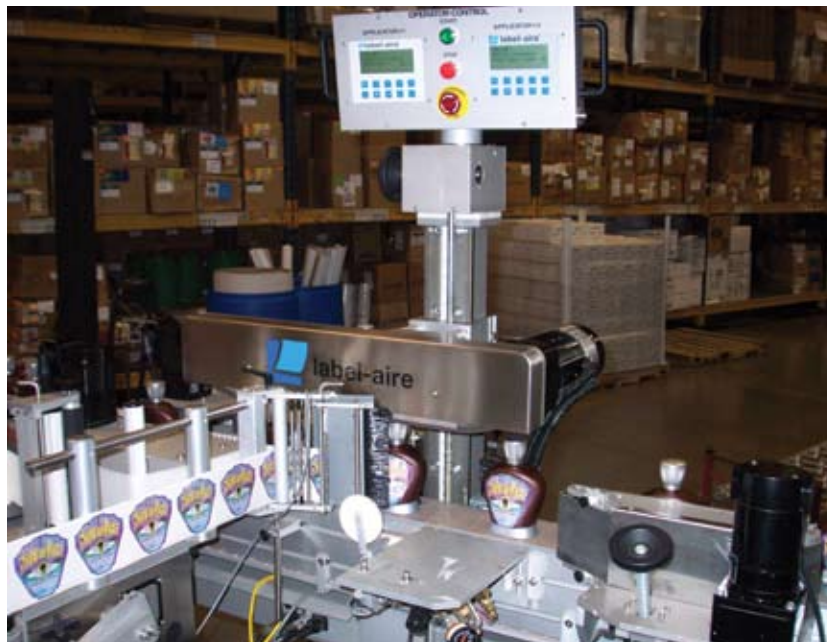
FRONT-AND-BACK LABELING. The rectangular bottle for which the labeler was originally purchased has been discontinued, but a switch to front-and-back labeling went off without a hitch.
